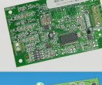
RX-16MF349 RADIO RECEIVER CARD, ALLOWS WIRELESS DEVICES TO BE ADDED. COMPATIBLE WITH 303, 433 & 915MHz DEVICES
